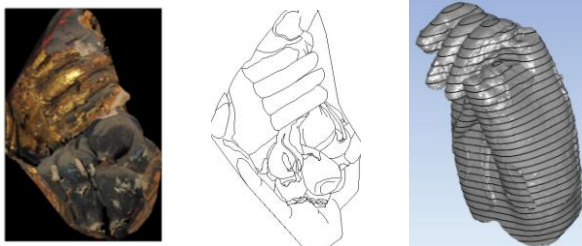
(a) Orthophoto map (b) digital line graph (c) contour map Figure 6 3D thematic maps
