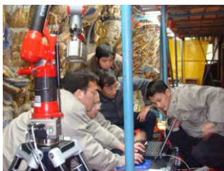
Figure 2 Data acquisition using Cimcore
