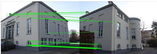
Figure 1. Repetitive texture patterns affecting the matching and leading to wrong correspondences.
