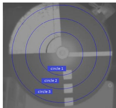
Figure 12. Thermometric image with readout circles
