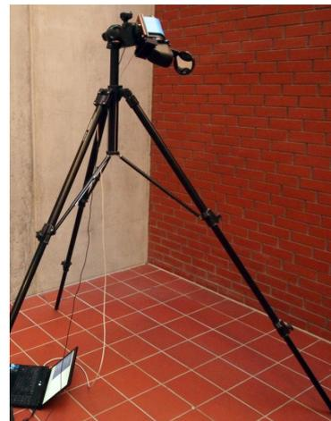
Figure 7. Practical test – scanner mounted on tripod
