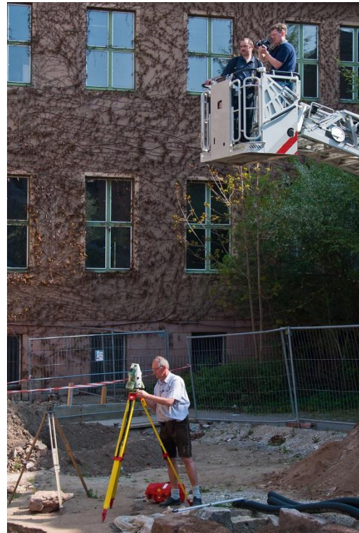
Fig. 4 Simultaneous total station and photogrammetric survey
