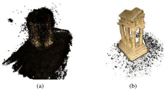
Figure 5: An example of photoconsistency volume (with color) before (a) and after (b) the spurious points removal.
