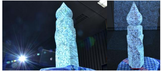
Figure 10: Photogrammetric acquisition of the white test object “Testy” using artificial texture from 3 video projectors.
