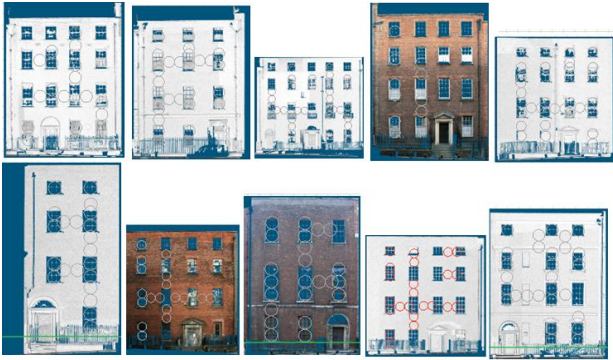
Figure 3. Testing classical proportions using orthographic imagery from surveyed classical buildings.
