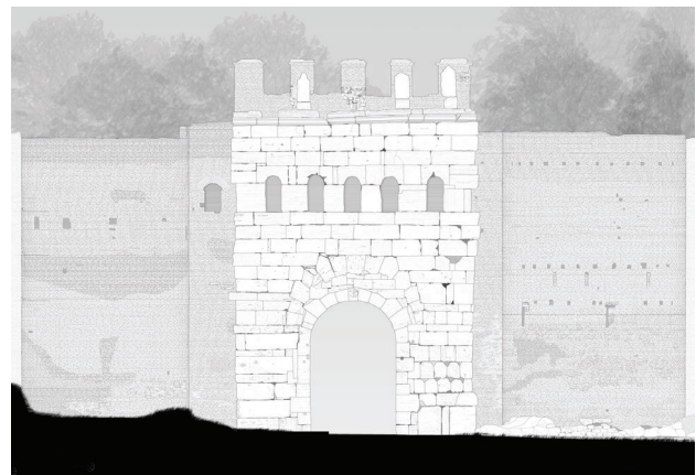
Figure 2. Porta Latina, 2012, geometric survey on photographic base ortho-rectified.
