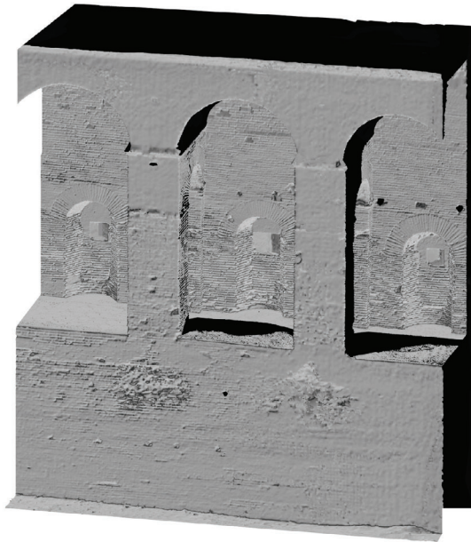
Figure 3. portion of 3D model: triangulated surface reconstruction.
