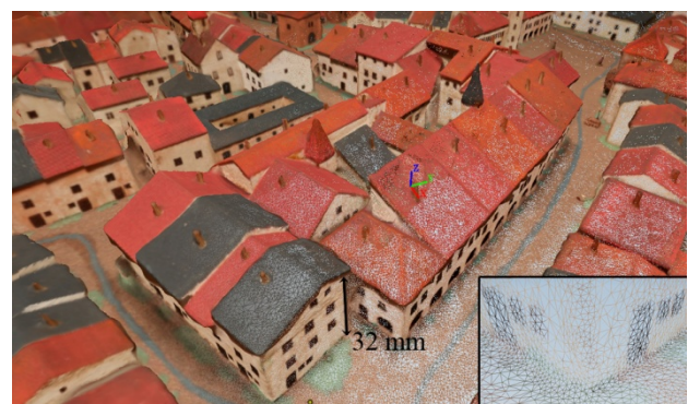
Fig. 4. 123D Catch results for the Epinal scale model
