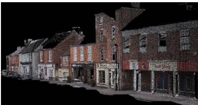
Figure 10. Point cloud data of buildings along the street
