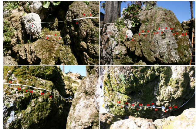
Figure 10. Digital photogrammetry to calculate the 3d position of the seismic tomography sensor
