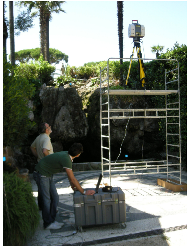
Figure 4. Acquisition data phases with laser scanner.
