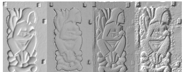
Figure 8: Visual quality check from left to right Carmine 1.09, Kinect, DCC and webcam with 123DCatch
