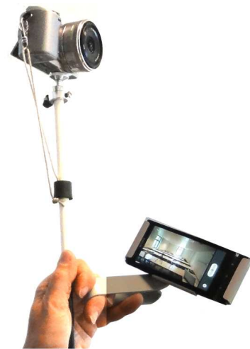
Figure 2. XLITE telescope staff with 3 rd generation SONY NEX-5R system camera WLAN capable camera with smart-phone(App) based remote control
