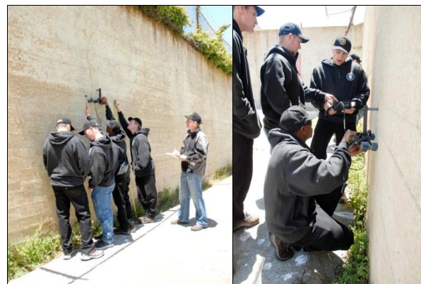
Figure 4. Chico State Students with Olson Instrument Engineer taking SASW measurements across a crack in the wall of the Rec Yard
