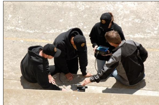
Figure 3. CSU Chico & Texas A&M University Students Learning to use Olson Instruments' Concrete Thickness Gauge
