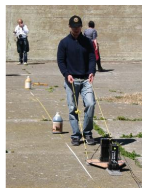
Figure 8. (left) GPR data acquisition in cross-dipole mode; (right) GPR survey geometry.
