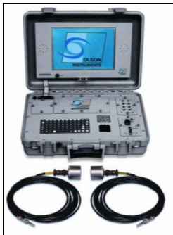
Figure 7. Olson Instruments' UPV and field ruggedized computer system
