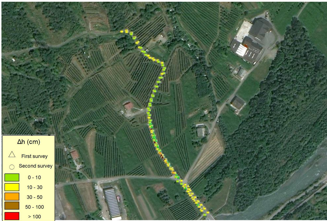
Figure 4. VT07 area: GNSS RTK results and differences with respect to HR DTM heights.
