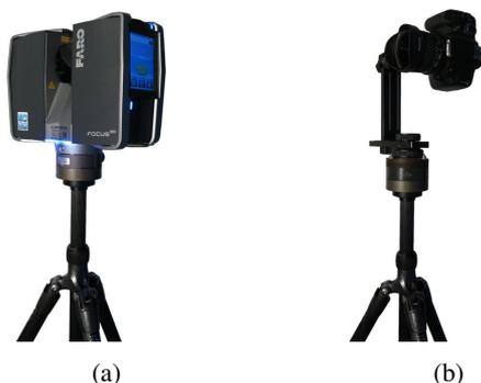
Figure 1: The data acquisition equipment: For range data acquisition, a Faro Focus 3D Scanner was used (a); additional color information was obtained using a customized adapter connecting the base tripod of the 3D scanner with a HDRI camera (b).
