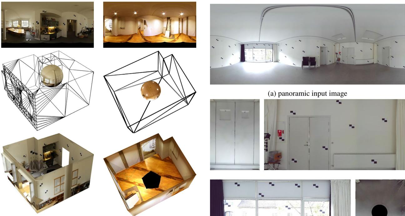
Figure 7: Two indoor scenes in different stages of reconstruction. The acquired high-resolution input panoramas (top row) were aligned to the geometry that was created from the laser range scan. The middle row shows the input geometry, and the aligned panoramic spheres. In the bottom row we see the same geometry using the generated orthographic views as textures, the ceiling has been omitted for a better visualization.
