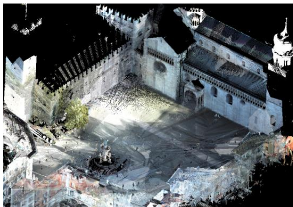
Figure 2. Close-up view of the coloured 3D point cloud collected by MMS in the Duomo square of Trento (Italy).
