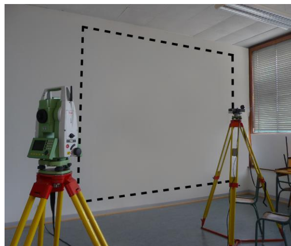
Figure 10. Depth calibration experiment (observed area in dotted lines)
