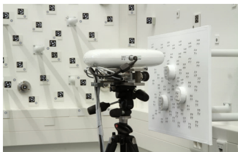
Figure 4. Calibration of the camera system with a reference object on a wall
