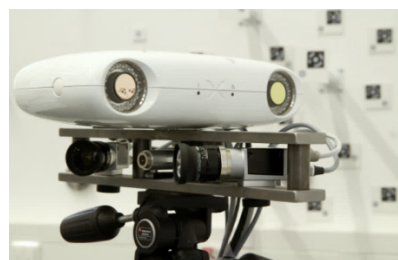
Figure 3. Measuring head: stereo laser-profile system (two Basler Ace cameras and laser line module) in the bottom and positioning component above (stereo camera system CamBar, AXIOS 3D services, white housing).
