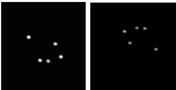
Figure 12. Left: Measuring image of a low-cost probe, Right: Measuring image of the toy drill probe with professional markers
