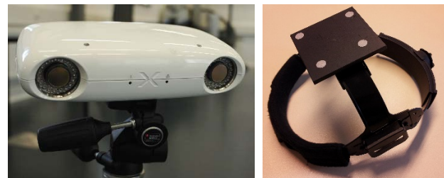
Figure 7. Left: AXIOS stereo camera CamBar B2, Right: light head belt with a targeted probe
