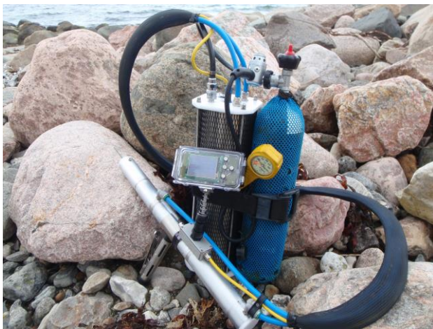
Figure 5. Diver held version of a device for assessing the state of preservation of waterlogged archaeological wood through the determination of wood density.
