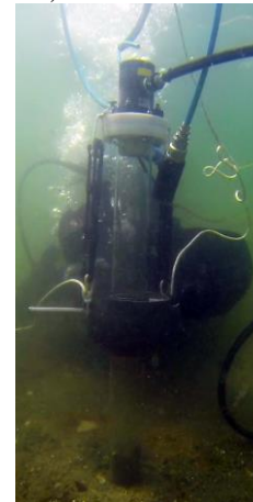
Figure 1. Core sampler. Vibracorer head uppermost with lead weight around the plastic coring tube to aid penetration of the seabed.
