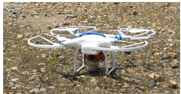
Figure 9. Mounting camera to UAV.
