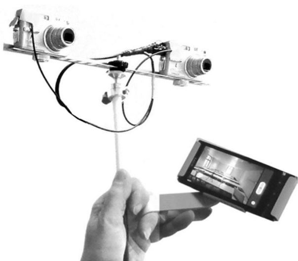
Figure 7. X-Lite carbon telescope staff carrying WLAN capable stereo-cameras with smartphone App based remote control (technical study, partly carried out by St. Kiel of the University of Appl. Sc. Magdeburg)
