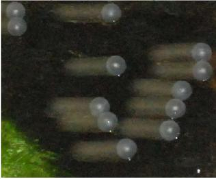
Figure 2 Deliberateley blurred targets for velocity determination
