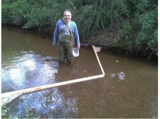
Figure 5 Two hinged wooden spas used for collecting spheres
