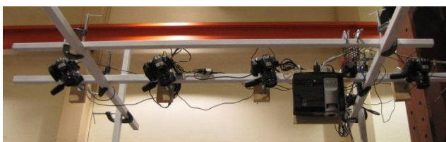
Figure 2. An example showing half the cameras and one of the projectors suspended from the support frame
