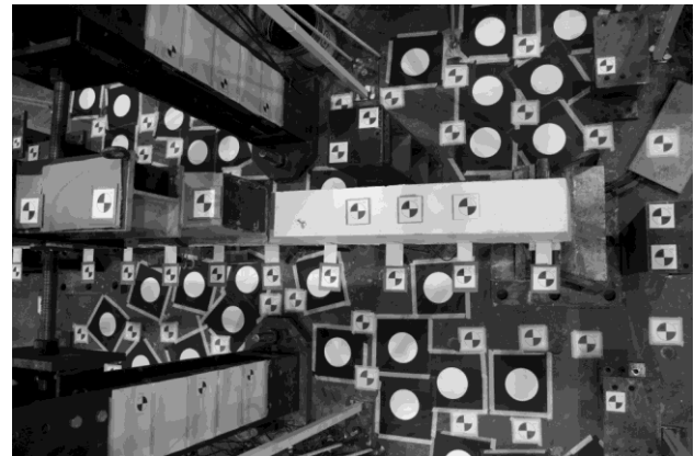
Figure 3. Distribution of physical signalized targets used for the exterior orientation estimation
