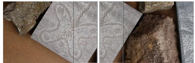
Figure 12: Typical pair of images acquired by the DSLR cameras of the scanner: The field of view of each camera is roughly  $23 \times 15$  cm. Considering the small overlapping region of 6.5 cm width (marked by a box in both images), this yields an overall footprint of the scanner of  $40 \times 15$  cm.
