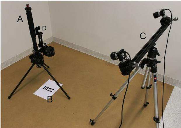
Figure 8: Setup for calibration of the T-shaped scanner structure: The scanner prototype A tracks a target B positioned in its field-of-view, and the external stereo camera rig C simultaneously tracks the target B and the white sphere D on the the scanner structure that is afterwards used to track the scanner position.
