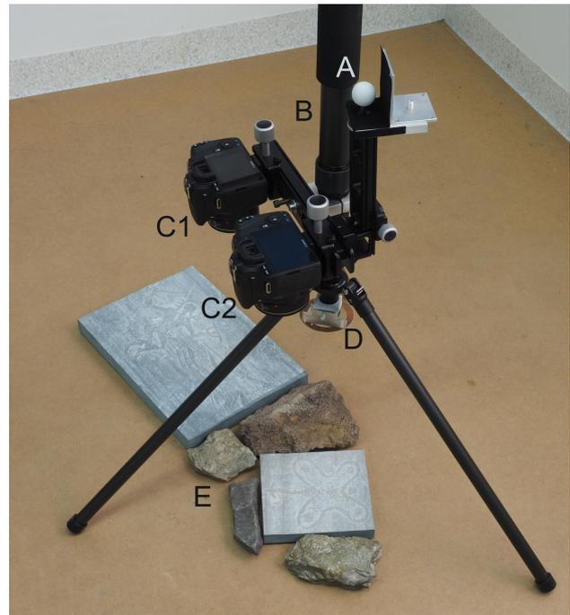
Figure 7: Scanner prototype used for data acquisition: A stereo rig containing two DSLR cameras (C1, C2) and a white sphere for outside-in tracking (A) are mounted onto a carbon fibre mount (B). A mount (D) is included to properly fix a detachable custom LED illumination component (not shown here). The scanner observes the laboratory mockup consisting of a few rocks and two 3D prints (E).
