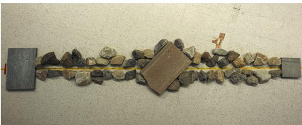
Figure 10: Test scene II as used for measurements to assess the drift of the reconstruction for larger rock panels: Two 3D prints of Valcamonica rock-art, a concrete plate and several rock samples are arranged to comprise a scene of roughly 250 cm by 50 cm.
