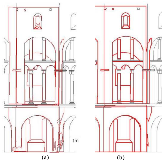
Figure 16. Superimposition of the final extracted sectional view (red) and the reference view (grey); a) result obtained without corrections; b) result obtained after manual corrections
