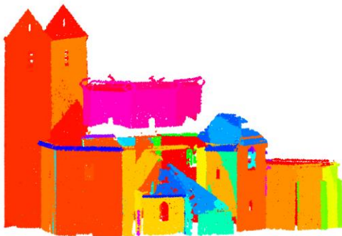
Figure 6. Segmentation results obtained for the point cloud of the exterior of the church (one color per entity)
