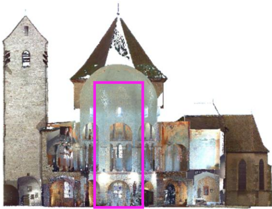
Figure 5. Point cloud of the expected sectional view (along west/east axis, seen from the south)
