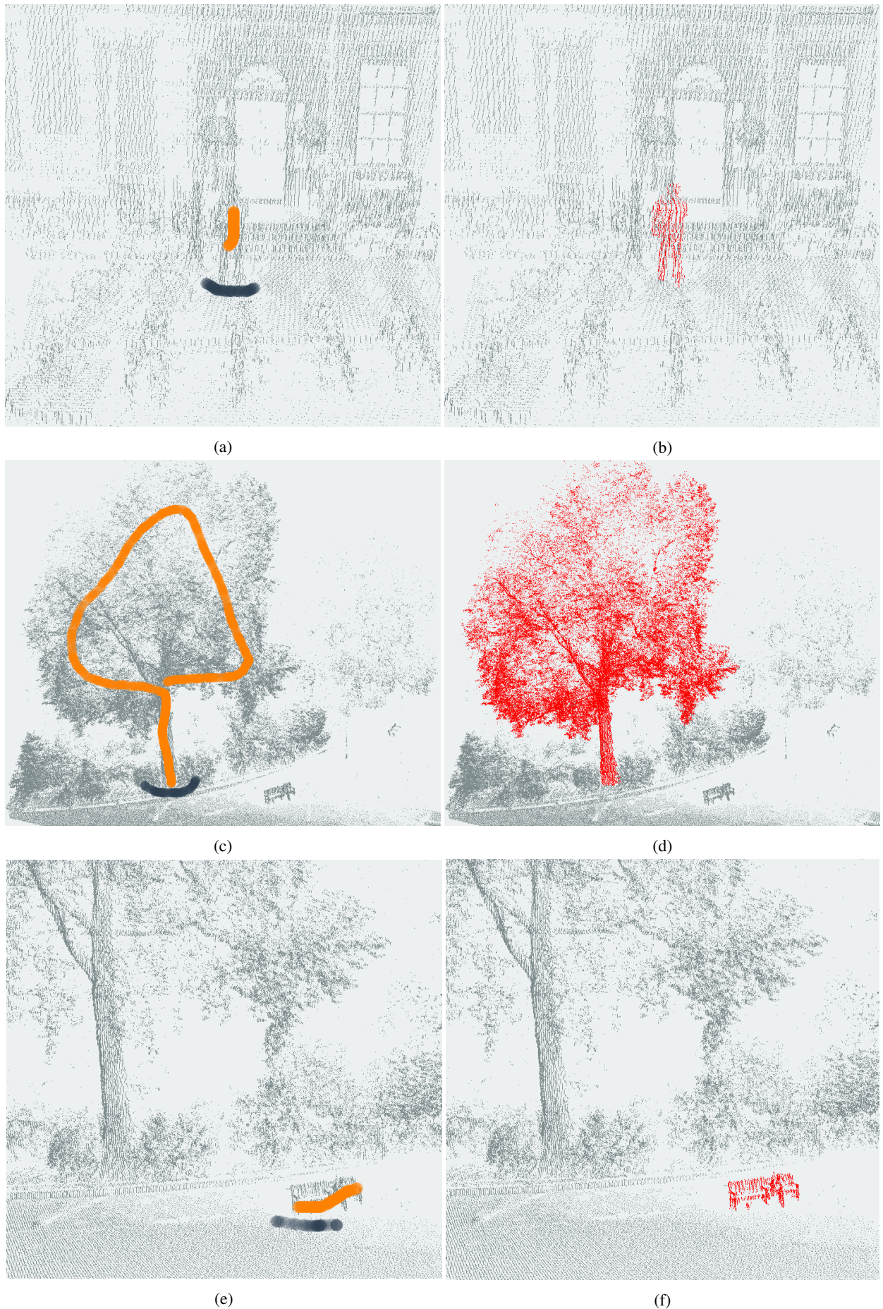
Figure 7: An illustration of segmenting person, tree and bench out from point clouds respectively: (a), (c), (e) in the left column show the user interactions and (b), (d), (f) in the right column display the corresponding results.
