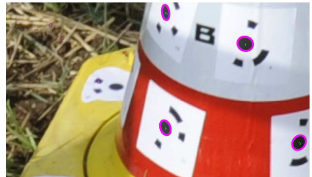
Figure 4: Image point coordinate measurement by ellipse fit.
