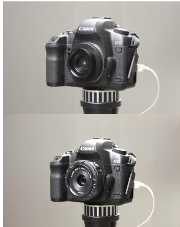
Figure 2. Pinhole optical system (top) and glass optical system (bottom)
