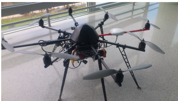
Figure 1. UAV platform equipped with 2D laser scanner Hokuyo and GPS.
