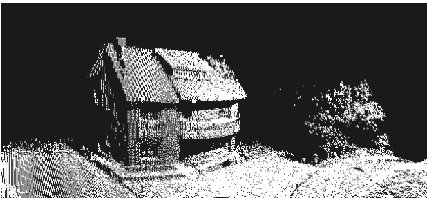
Figure 5. Example of point cloud acquired by the UAV system with 2D laser and GPS following methodology 2: combined acquisition of façade and roof.
