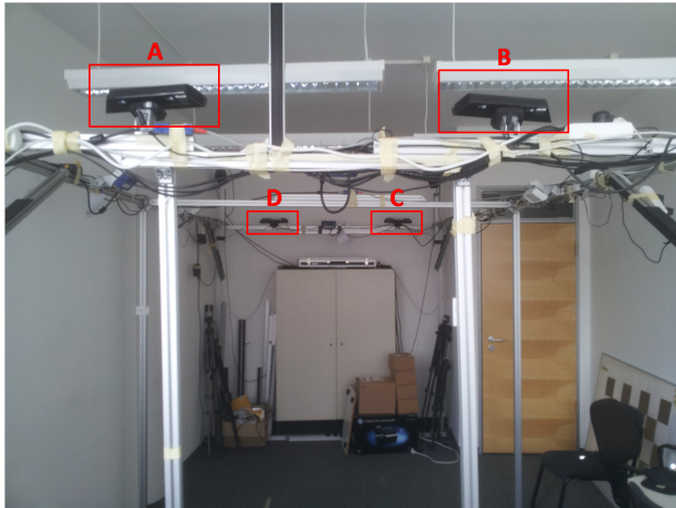
Figure 2: Aluminium construction with mounted Kinects sensors
