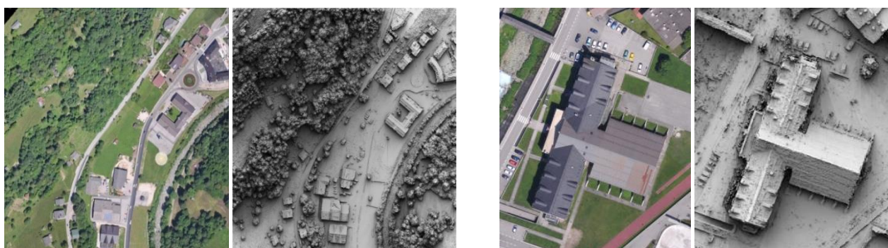
Figure 4: An example of the photogrammetric DSM (shaded view) over an alpine village (left) and a closer view of a building (right).
