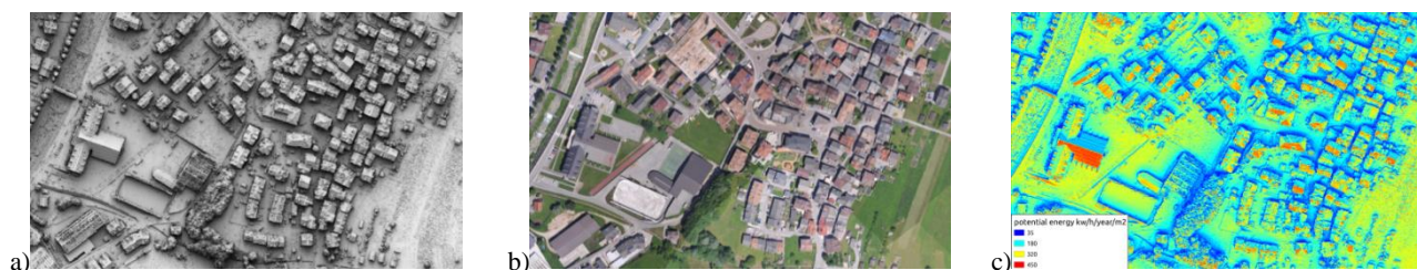
Figure 1. Results of the photogrammetric DSM generation from aerial images (a), true orthophoto (b) and solar potential energy estimation visualized with the raster-based webGIS tool created within the 3DSolarWeb project (c).
