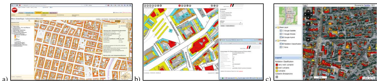
Figure 2: Examples of data representations by means of WebGIS for solar cadastres and photovoltaic potential of buildings: reclassified rasters of global solar irradiance overlaid to cadastral maps (Vienna – a), vector roof facets with assigned averaged values of incoming solar irradiance (St. Gallen – b), reclassified raster of PV potential overlaid on an orthoimage (Brixen – c).
