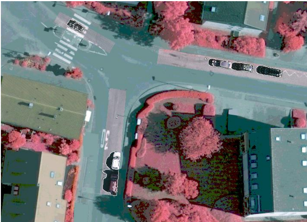
Figure 6a. This is the result after applying filtering on the image. The algorithm couldn't distinguish between the vehicle and its shadow.
