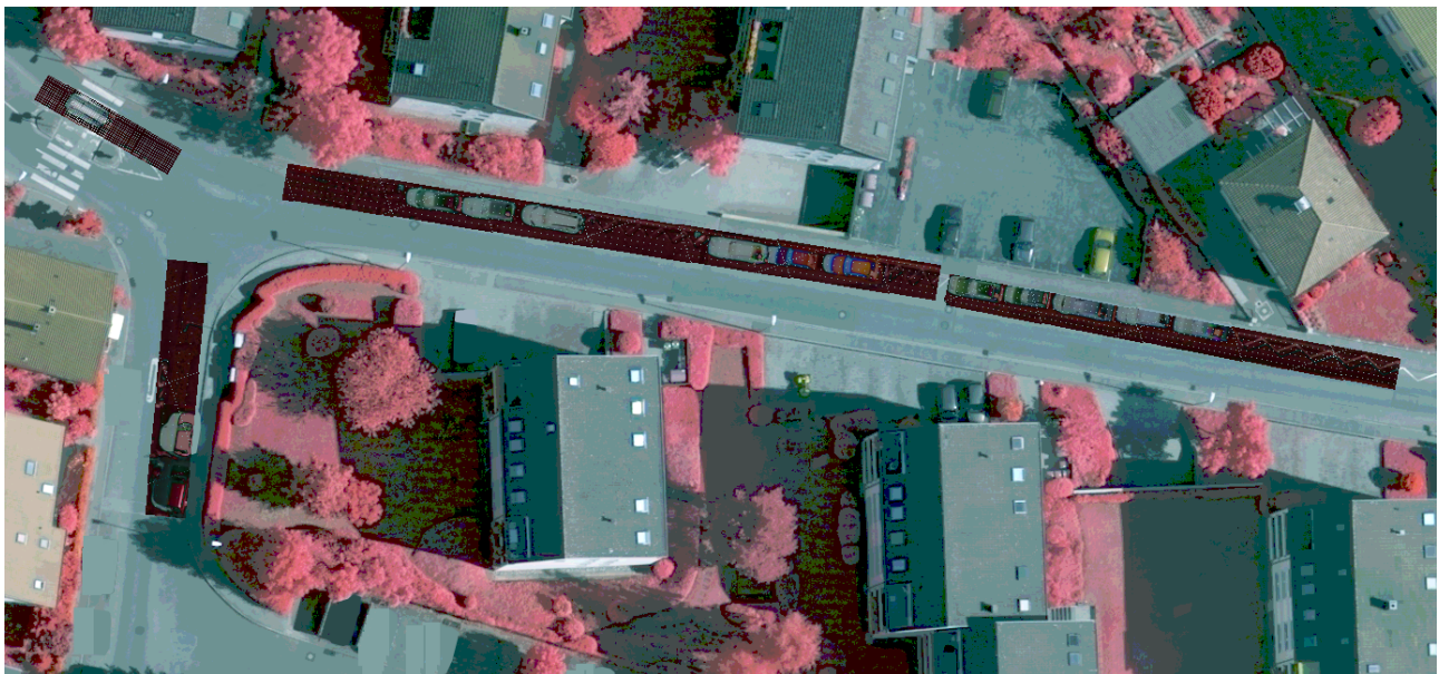
Figure 5. This is the result after registering the target image on the source image. Vehicle on the road can be recognised clearly.
