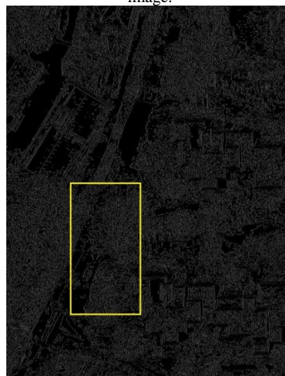
Figure 2. This figure shows the outline of image segmentation on the original image after converting the original image to greyscale. The area in the yellow box is part of road that is in the shadow. As it can be seen the vehicle in the shadow is not recognisable.
