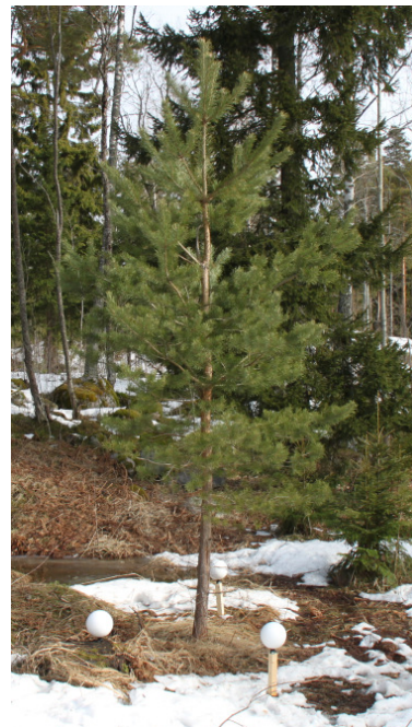
Figure 1. The pine sample before the measurement in April 2013. The white spherical reference targets visible in the image were used for the co-registration of scans.
