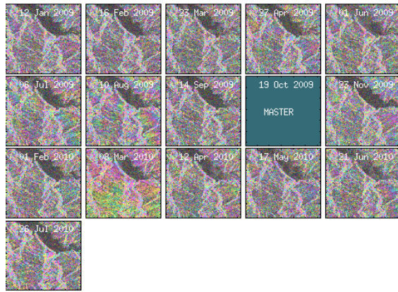
Figure 4. Interferograms for the Tehri region. The image acquired on 19th October 2009 is chosen as the master image.
