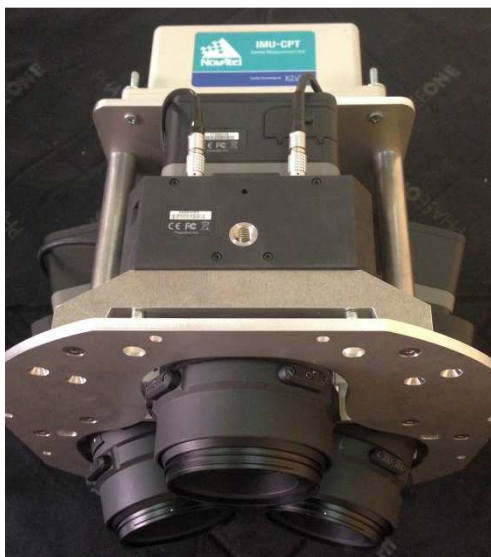
Figure 1: setup of a camera-triple with GNSS-INS
