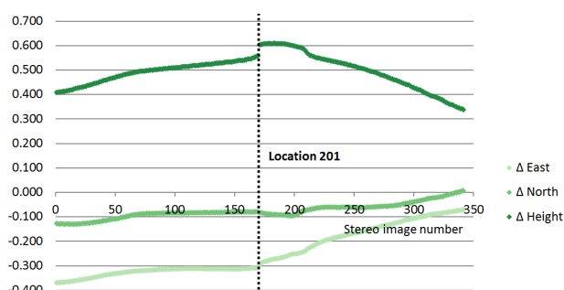
Figure 10. Deviations of projection centers for sequence 2.1
