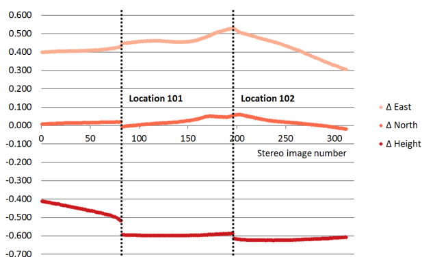
Figure 8. Deviations of projection centers in m for sequence 1.2
