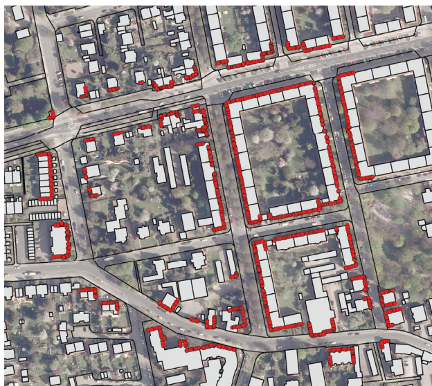
Figure 2. Test area in Hannover, Germany, with an area of 300 m x 300 m. Orthophoto overlaid with building footprints (gray area), road boundaries (black lines) and measured facade points (red dots).
