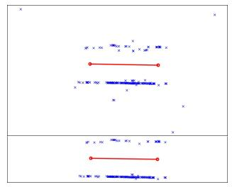
Figure 5. Plan view of automatically reconstructed points of a stereo pair: initial points (above) and after 3D filtering (below).
