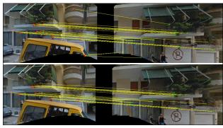
Figure 4. Outlier removal by filtering out deviating line slopes.
