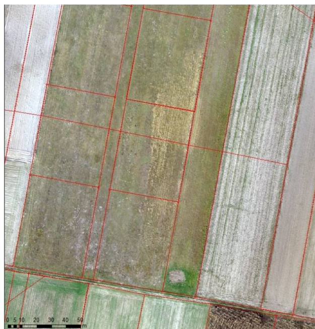
Figure 7. An example of discrepancies between boundaries existing in the cadastre and real land-use conditions detected on the basis of products from the UAS platform
