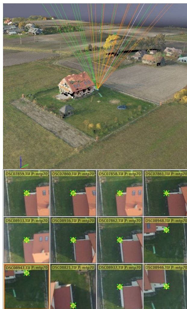
Figure 6. An example of an intersection with the use of the multi-photo measurement method
