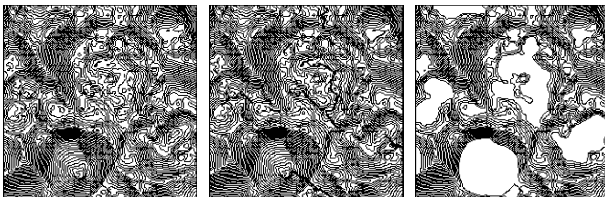
Figure 4. Relief with contour lines, Biokovo DTM5 (left - a), after the pit removal by carving method (middle - b) and after the pit removal by filling method (right - c)
