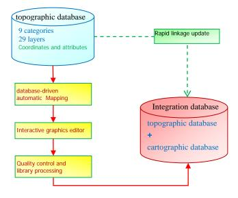
Figure 4. The technology methods and steps of integration cartographic database establishing
