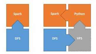
Figure 3: comparing the schematics of direct data import into Sark from a Distributed File System (DFS) versus sideloading via a Virtual local File System (VFS) and Python.
