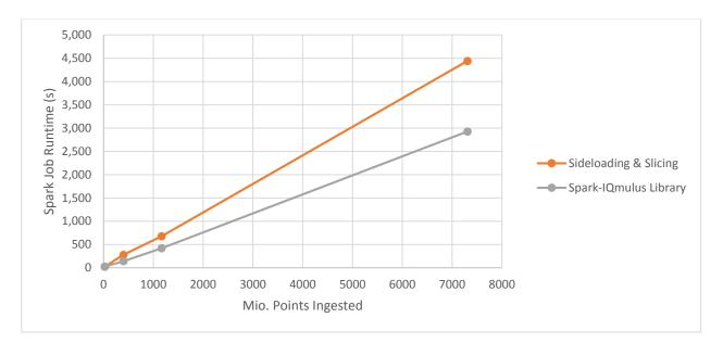
Figure 11: Runtime for sideloading of a large sized point cloud data set over varying number of points.
