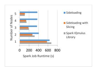
Figure 8: Effect of varying the number of nodes for a fixed sized point cloud.
