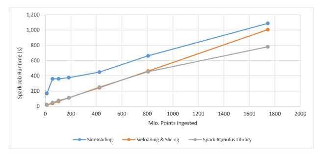
Figure 9: Runtime for sideloading over varying number of points from a medium sized point cloud data set.
