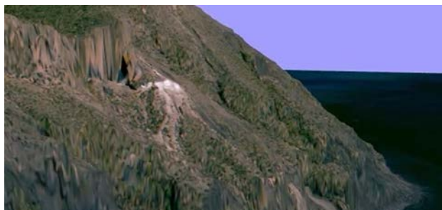
Fig. 10: DOP Luting due to steepness in a 3D visualization of a DOP
