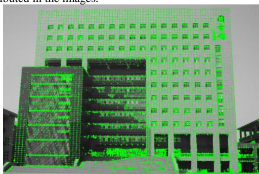
Figure 9. Corner points extracted from the camera image
