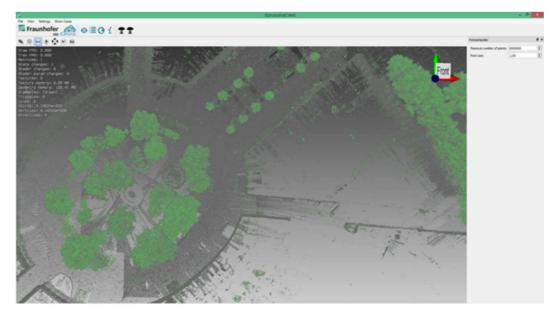
Figure 8. View on the Toulouse data set during asynchronous refinement. Note the difference in point density between the left and right parts of the image.
