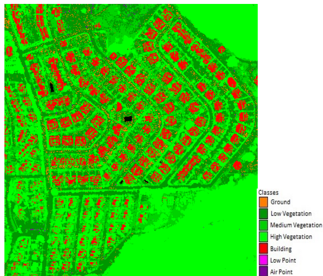
Figure 5. The roughly classified points cloud of the test area with standard parameters.
