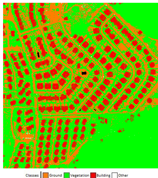
Figure 6. The classified points cloud of the test area with Approach 1 (with spatial-based and echo-based features).
