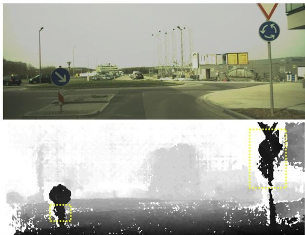
Figure 1. Example of SGM failure at object borders in front of a uniform background. Pixel intensities range from near to far from dark to bright. Pixel without disparity value (invalid disparities) are white.
