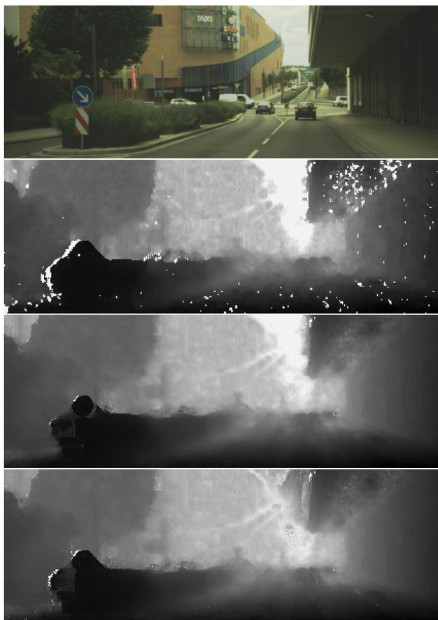
Figure 3. Picture detail of traffic scene. From top to bottom: Left color image, SGM image, output of basic variant (10 IVs, threshold=0.1), output of feedback variant (5 IVs, threshold=0.07). Note the contours of the sign on the left hand side
