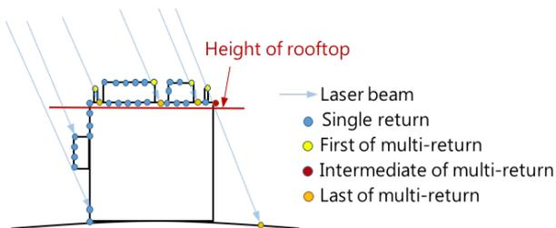
Figure 6. The concept of selecting laser points above the height of rooftop.
