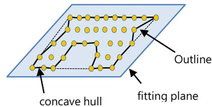
Figure 7. The illustration diagram of concave hull and outline of a cluster points
