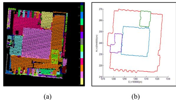
Figure 8. An example of extracted building outline and structure lines: (a) the image of segmented point clusters of the roof points; (b) the results of extracted boundary lines.
