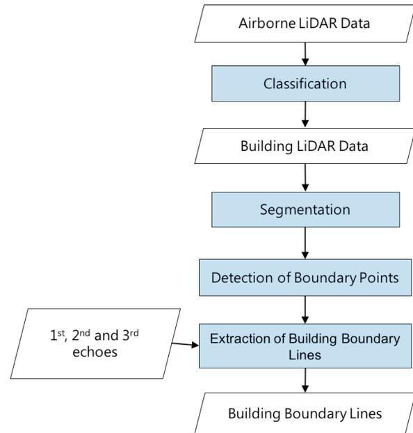
Figure 4. Flowchart of data processing of the proposed algorithm.
