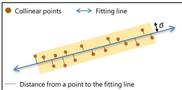
Figure 10. The conceptual illustration of the proposed line fitting process.
