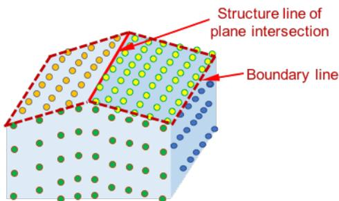
Figure 3. Characteristics of LiDAR point distribution and the the proposed approach to boundary extraction.
