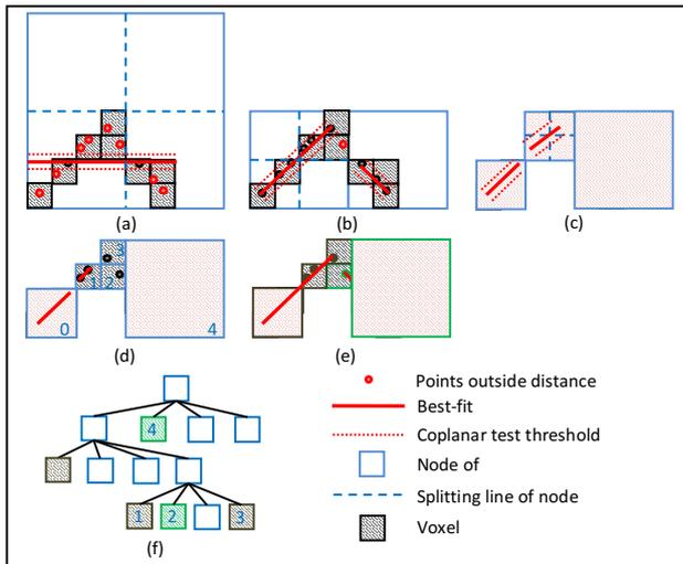
Figure 5. Split-and-merge segmentation for point group of the gable roof. (a)-(d) Splitting process; (e) results of merging process; (f) tree representation (using a quadtree for simplicity).
