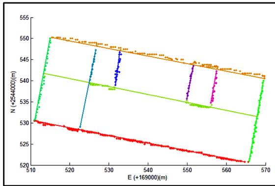
Figure 9. An example of extracted 2D lines by using Hough transform.
