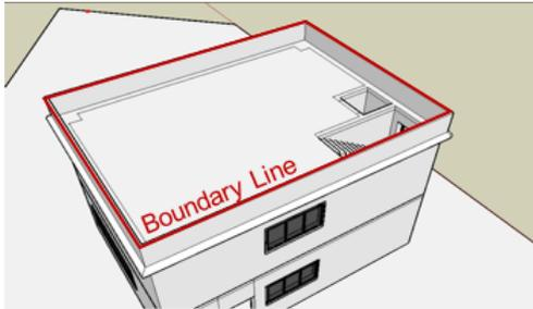
Figure 2. Appropriate boundary lines of a building with parapets on the roof.
